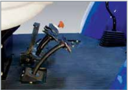
Live PTO with Dual stage clutch Allows gear and ground speed changes without affecting PTO RPM
