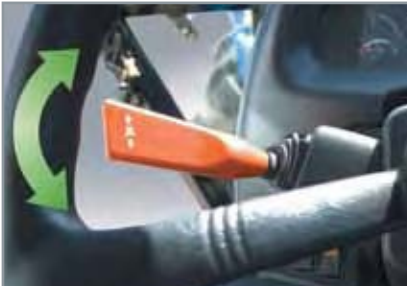
Power Shuttle Lever (optional) Maximizes ease of use with effortless, clutch-less directional changes
